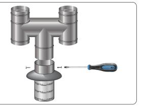
2. Push the barbed section into the twin wall flue, using protective gloves.
